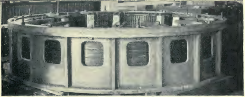
FIG. 93.—Core ready Assembled and under Pressure. Adolf Ungers Industria Aktiebolaget.
